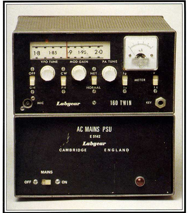
The Labgear 160 Twin 'phone/CW transmitter for 'Top Band' (1.8 – 2Mc/s)
